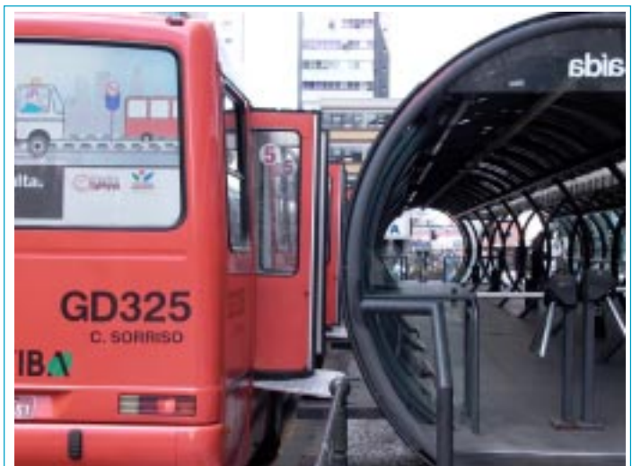
A Curitiba bi-articulated bus stops at a “tube” passenger station. Ramps extend both ways to facilitate and expedite the passengers’ entrance and exit from the five-door vehicles.
